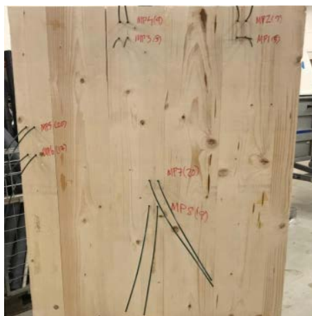
Figure 6.4-1 Example of instrumentation with probes at various depths and positions on a test piece of a floor element. Courtesy of F. Herrmann.
