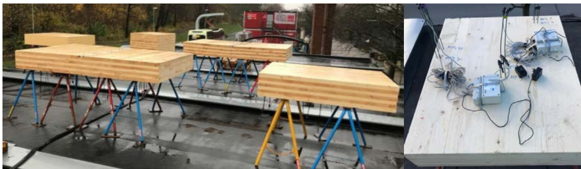
Figure 5.7-1 Test setup for outdoor floor elements. Tests performed by Herrmann. To the left is the exposed samples and to the right the automatic measurement devices installed at different depths (Herrmann, with permission).
