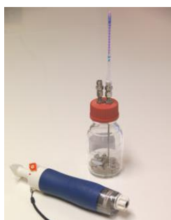
FIG 2. Set-up to measure NH 3 on detection tube
